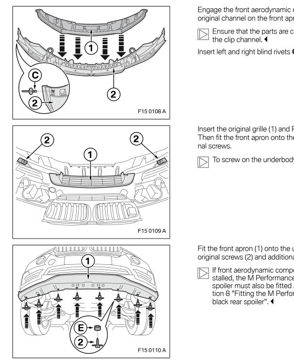
Engage the front aerodynamic components (1) in the original channel on the front apron (2).
