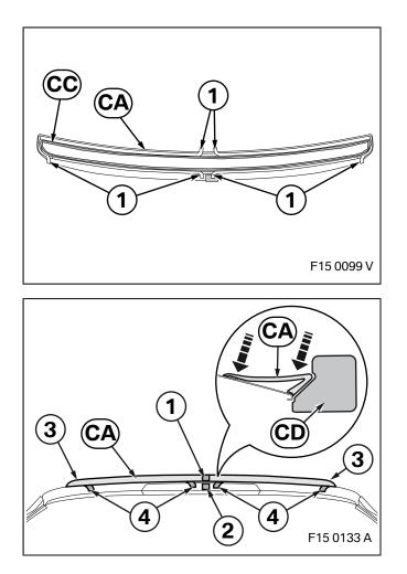
Remove the adhesive backing films on rear spoiler **CA** just enough to form small tabs (1).
