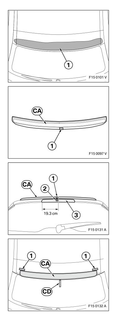
The areas being bonded (1) must be completely dry, clean and free from wax or grease.
