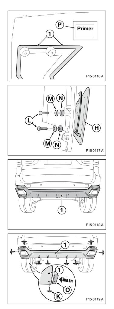
To install side flaps **H**, the areas (1) (not grained) must be cleaned and pre-treated with primer **P**.
